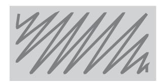
We recommend Soudall Contact adhesive is used and that the glue is piped across the back of the panels like this to create a good bonding surface.
