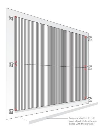
For large panels or if layering panels above one another we also recommend air nails / nail gun is used in the four corners for extra stability and that a temporary batten is installed at the base on the panels to take the weight whilst the adhesive dries.
